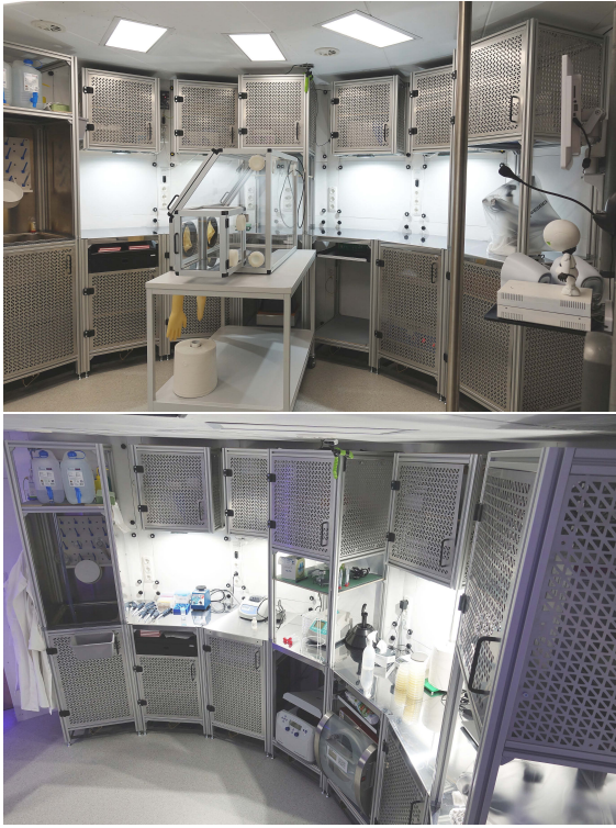
Figure 6: Photo of part of the laboratory module interior with seven racks: full-size water and storage racks, four bench-size racks and hanging racks forming two work spaces. Depth perception camera is visible in the top middle of the photo, aiming at the opposite line of racks between doors 1 and 2.
